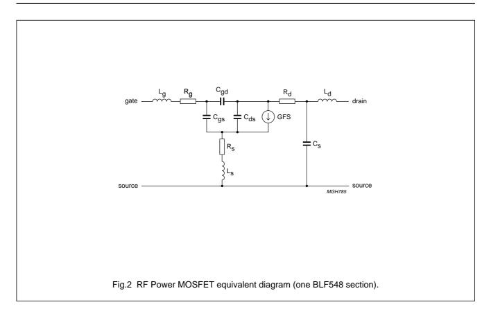
At the following pages the design steps are presented which were followed at PHILIPS' laboratories in order to design a 150 W unit. Using the diagram shown in Fig.2, powergain and impedances have been calculated first, using the data given in Table 2.
